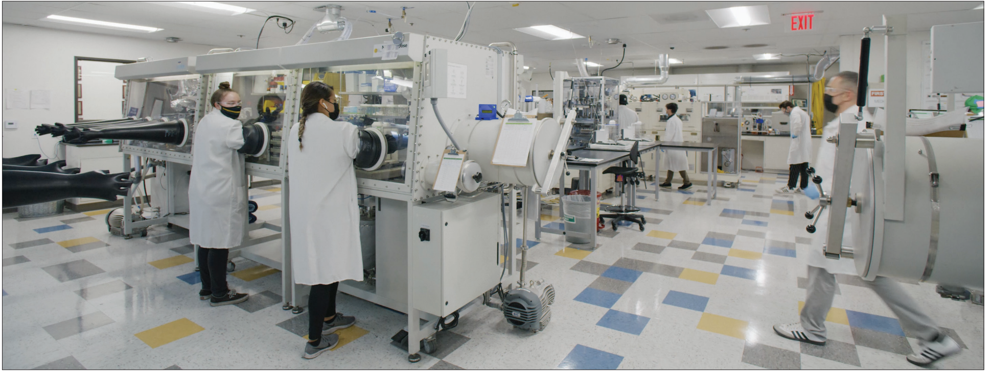
The Wildcat Discovery Technologies technicians are shown working in glove boxes that create a sterile environment. Photo courtesy of Wildcat Discovery Technologies
